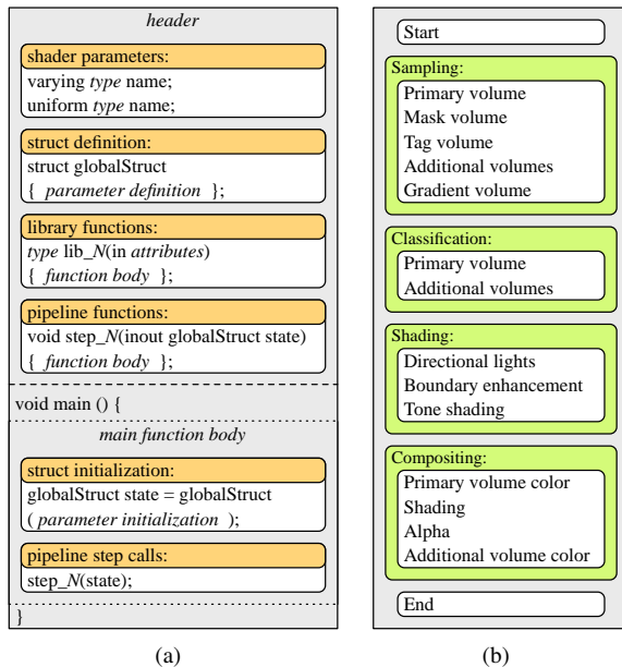
Figure 4: (a) Overview of the composed SuperShader code of the pipeline with library and pipeline function. (b) The 16 pipeline steps are grouped in four main rendering steps.
